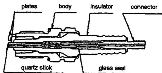
Figure 18. Fiber optic sensor integrated with spark plug [1]
