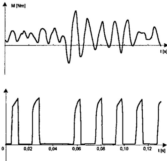
Figure 11. Torque and ignition signals for 3500 rpm, throttle 75%, 1 misfire [6]
