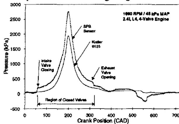
Figure 15. SPB Sensor and Kistler 6125 Signals Plotted as a Function of Crank Position for One Combustion Event at Part Throttle [12]
