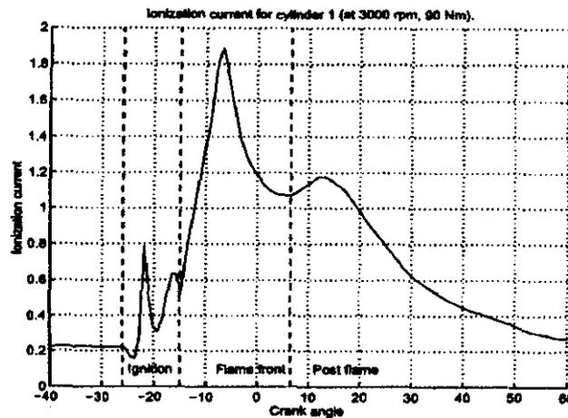
Figure 8 An ionization signal showing the three phases: ignition, flame front, post flame [7]
