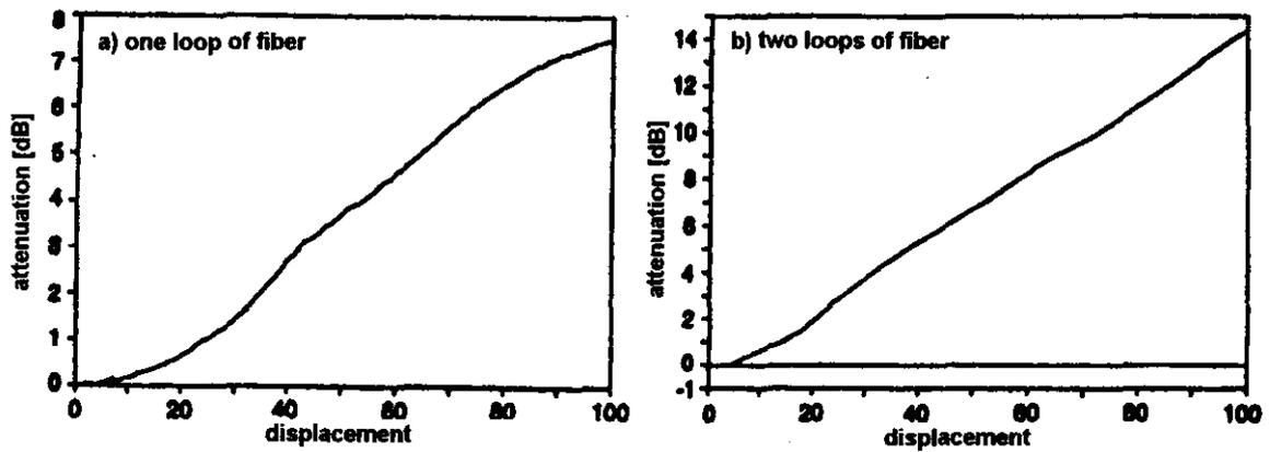
Figure 20. Magnitude function of the fiber optic sensor [18]
