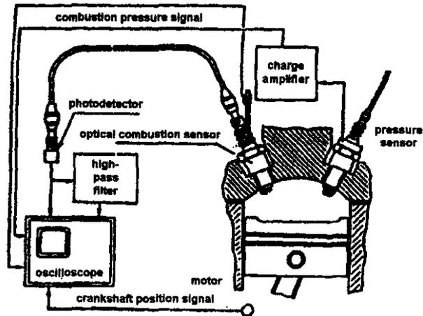
Figure 17. Schematic diagram of an Engine Combustion Investigation System
