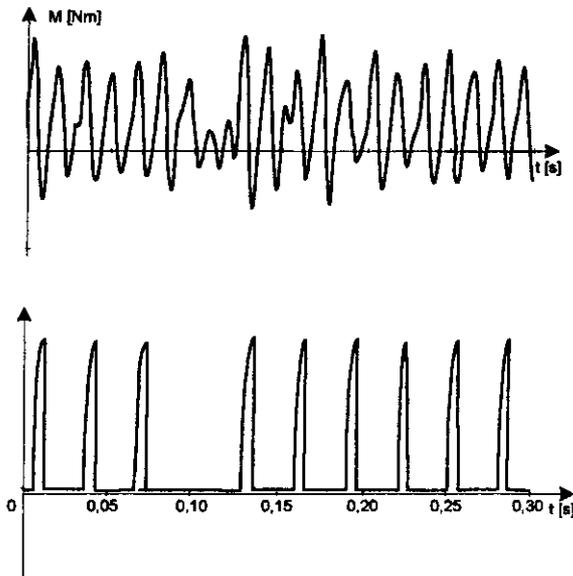
Figure 10. Torque and ignition signals for 2000 rpm, throttle 100%, 1 misfire [6]
