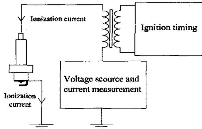
Figure 7 Measurement of the ionization current
