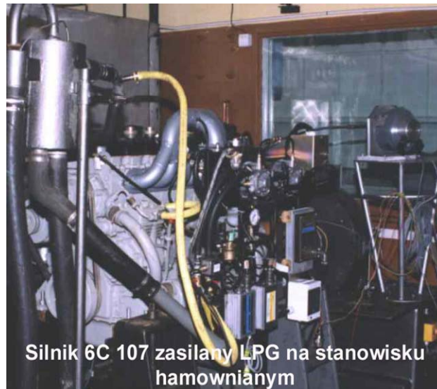
Rys.2. Silnik 6C107 na stanowisku hamownianym Fig. 2 Engine 6C107 mounted at braking device station.
