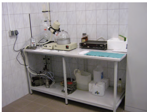
Fig. 5. The equipment for safe, evaporative concentration (by vacuum distillation) of \text{H}_2\text{O}_2 low concentration solutions (authors)
