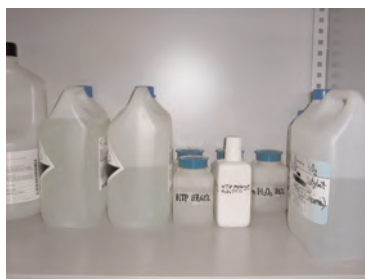
Fig. 2. Row solutions (low concentration), samples of HTP (87,6%) and concentrated (stabilized, 86%) H 2 O 2 prepared with the use of special vacuum rotary evaporator by the authors
