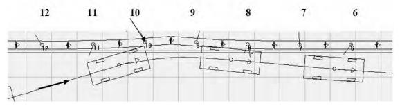
*Fig. 4.* The position of the barrier hit by the vehicle at a 16 degrees angle, vehicles centre of inertia trajectory and vehicle contours at 0.5 s intervals. The visible part of the barrier consists of segments 6-12
