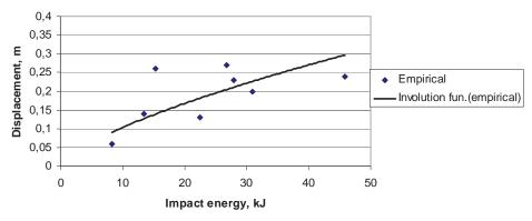
Fig. 6. Experiment results in study [10] and an approximation of the results
