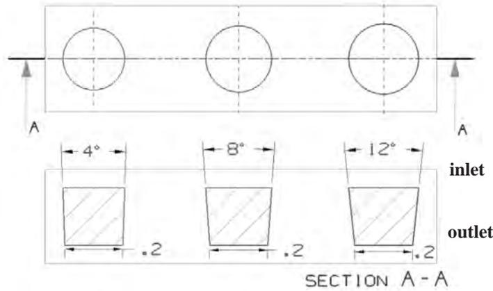
Fig. 2. Types of axial holes geometry (All dimensions are in inches)
