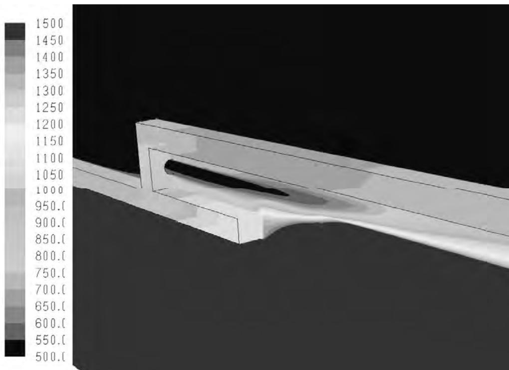
Fig. 8. Final model Axial hole cross section temperature [between 500K and 1500K]
