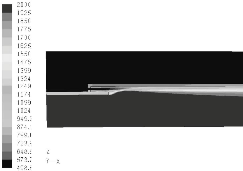
Fig. 7. Final model axial hole cross section temperature [max 2000K]
