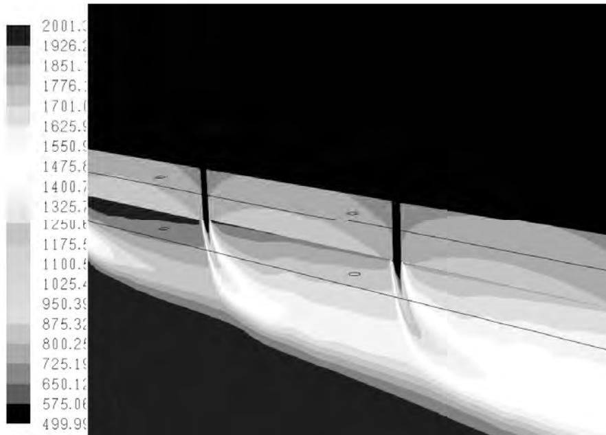
Fig. 11. Final model multiholes cross section temperature [max range, close view]
