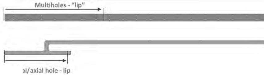
*Fig. 14. Areas from which temperatures were read - liner lip (from the hot side) - all cases*
