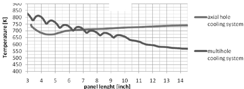
*Fig. 17. Temperature plots on liner panel (from the hot side) all cases*
