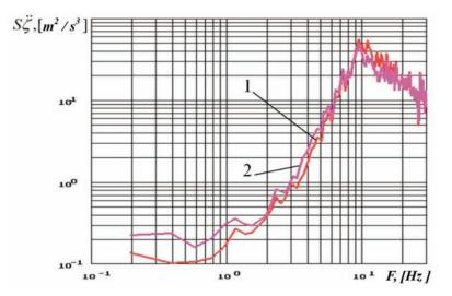
Fig. 7. Spectra of vertical speedups of the left swivel member of a front suspension: 1 - a regular suspension MSV = 29.41 m/s<sup>2</sup>, 2 - a semiactive suspension MSV = 29.38 m/s<sup>2</sup>
