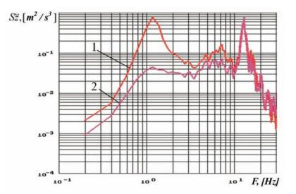
Fig 6. Spectra of vertical speedups of a body over a rear suspension: 1 - a regular suspension, 2 - a semiactive suspension
