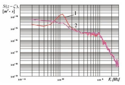
*Fig. 9. Spectra of relative conveyances of a front left pneumospring: 1 - a regular suspension MSV =0.0131 m, 2 - a semiactive suspension MSV =0.0106 m*
