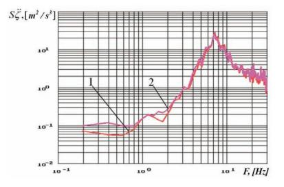
Fig. 8. Spectra of vertical speedups of the rear bridge: 1 - a regular suspension  $MSV = 12.71 \text{ m/s}^2$ , 2 - a semiactive suspension  $MSV = 13.16 \text{ m/s}^2$
