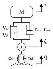
Fig. 1. One-basic two-mass model of a suspension with a controllable damper and a controllable pneumatic spring: M, m – cushioned and uncushioned masses,  $Z, \zeta$  – vertical displacement of cushioned and uncushioned masses; q kinematic fluctuation,  $c_{sh}, r_{sh}$  – rigidity and coefficient of resistance of the tyre,  $V_0, V_d$  - the basic and additional volumes of the pneumatic spring,  $r_{min}, r_{max}$  - the min and max values of damper resistance coefficient
