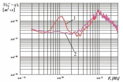
*Fig. 10. Spectra of relative conveyances of the front left tire: 1 - a regular suspension MSV =0.00637 m, 2 - a semiactive suspension MSV =0.00634 m*
