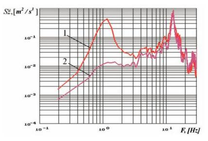
Fig. 5. Spectra of vertical speedups of a body over a front suspension: 1 - a regular suspension, 2 - a semiactive suspension
