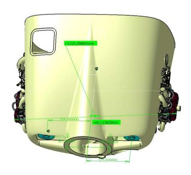
Preliminary analysis of CEPU power system configuration on the I-23 plane – Two Rotax 914F engines (2 x 115 HP), compared to the shield of actual single engine (Lycoming 360)
