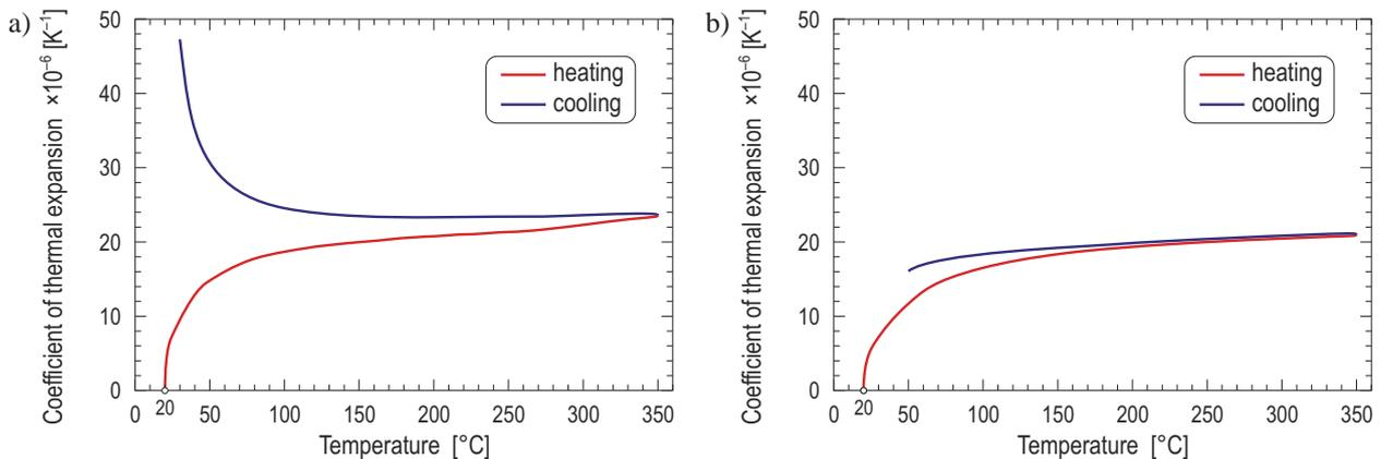
Fig. 5. Changes in coefficient of thermal expansion for the PA12 aluminum alloy (a) and the new composite material (b)
