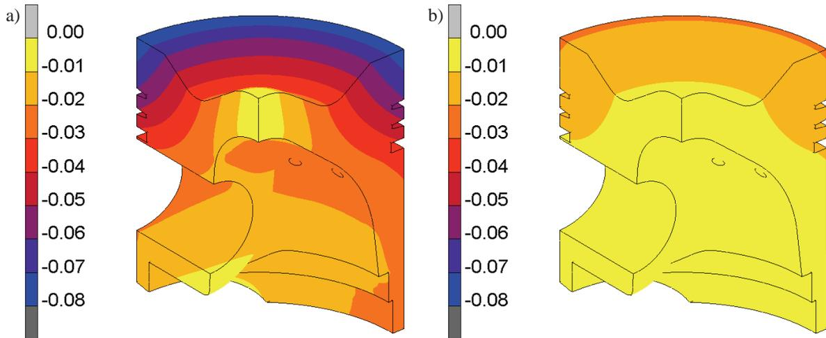
Fig. 8. Contour bands of the radial displacement [mm] for the piston made of standard material (a) and the new composite material (b) after cooling it to the temperature of 50°C
