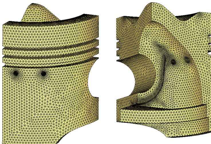
*Fig. 4. FE model of the quarter of the piston*
