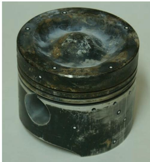
Fig. 1. A view of the piston of the S12U engine. Some markers used during a 3D laser scanning are visible
