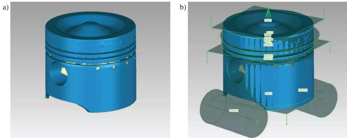
*Fig. 2. A scan view of the piston (a) and selected geometrical objects matched to the cloud of points (b)*
