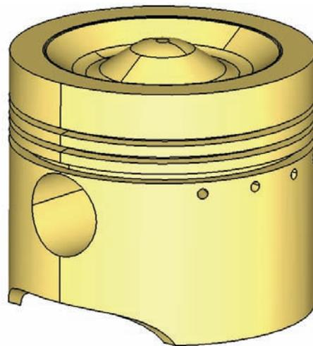
*Fig. 3. A geometrical model of the piston*
