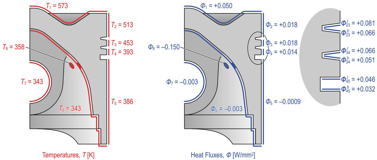
Fig. 6. Average values of the thermal boundary conditions for the S12U engine piston, according to [1–3]
