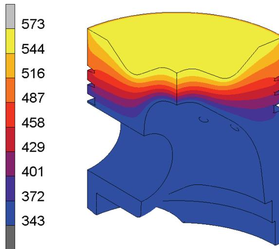
Fig. 7. The temperature contour bands [K] for the piston under thermal load
