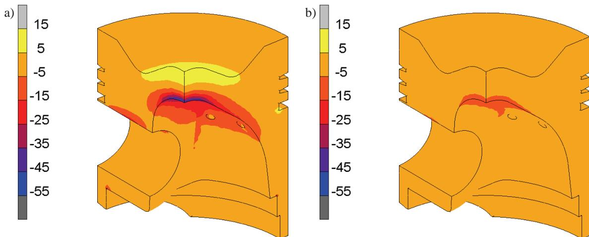
Fig. 9. Contour bands of the radial stress [MPa] for the piston made of standard material (a) and the new composite material (b) after cooling it to the temperature of 50°C
